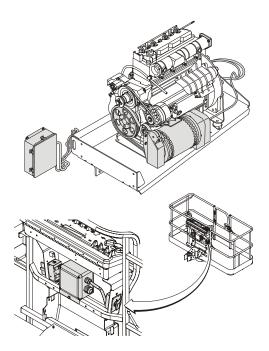
The SkyPower™ system supplies AC power to the platform through an AC receptacle to run tools, lights, cutting, and welding equipment.
