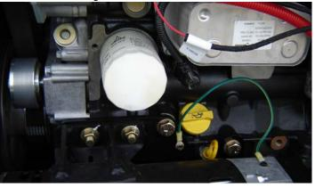
Lube Point(s) - Fill Cap/Spin-on Element Capacity - 9.6 Quarts (9.0 L)
