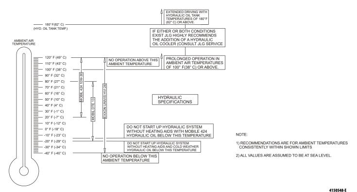
Figure 7-5. Engine Operating Temperature Specifications - GM - Sheet 2 of 2
