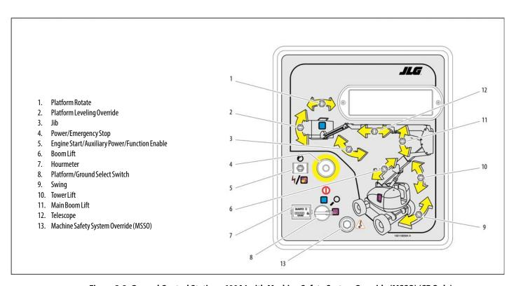
Figure 3-2. Ground Control Station - 600AJ with Machine Safety System Override (MSSO) (CE Only)
