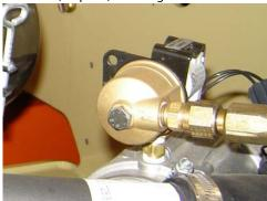
Interval - 3 Months or 150 hours of operation Comments - Replace filter. Refer to Section 7.6, Propane Fuel Filter Replacement
