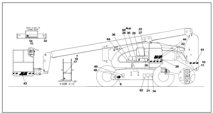
Figure 4-11. 600A & 600AJ Decal Installation - Sheet 1 of 4
