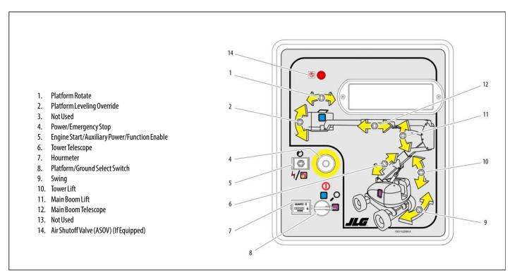
Figure 3-3. Ground Control Station - 600A
