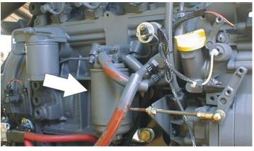
On Engine: Lube Point(s) - Replaceable Element Interval - Change in accordance with engine manual
