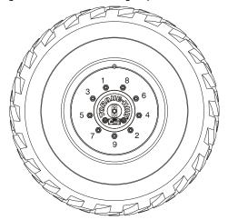
**3.** The tightening of the nuts should be done in stages. Following the recommended sequence, tighten nuts per wheel torque chart.
