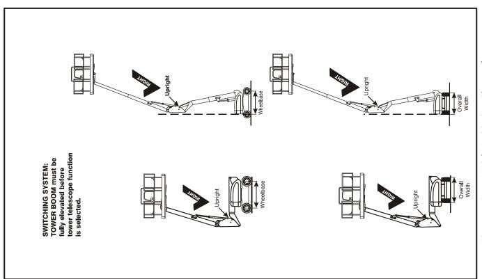
Figure 4-6. Boom Upright Positioning - Sheet 1 of 2
