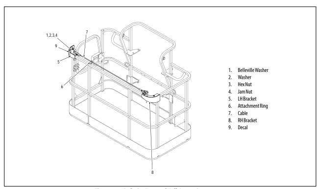
Figure 6-2. Bolt-On External Fall Arrest System
