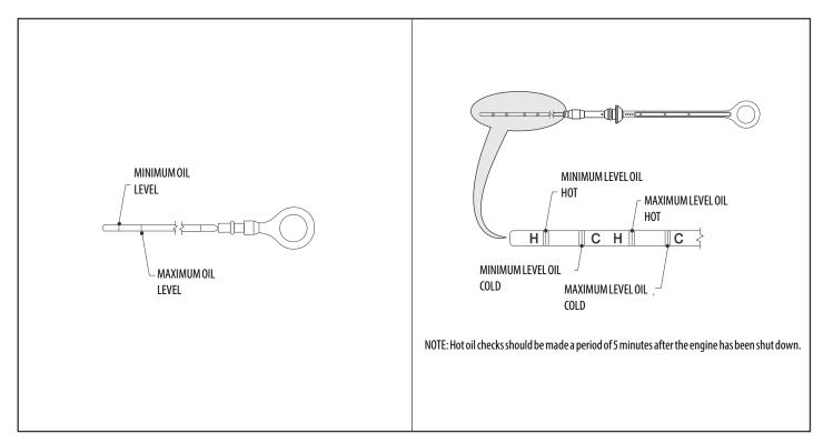
Figure 7-9. Deutz 2011 Engine Dipstick
