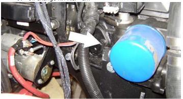
Lube Point(s) - Fill Cap/Spin-on Element Capacity - 4.5 qt. (4.25 L) w/filter Lube - EO Interval - 3 Months or 150 hours of operation Comments - Check level daily/Change in accordance with engine manual.
