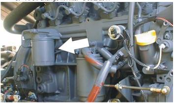
Lube Point(s) - Fill Cap/Spin-on Element Capacity - 11 Quarts Crankcase; 5 Quarts Cooler Lube - EO
