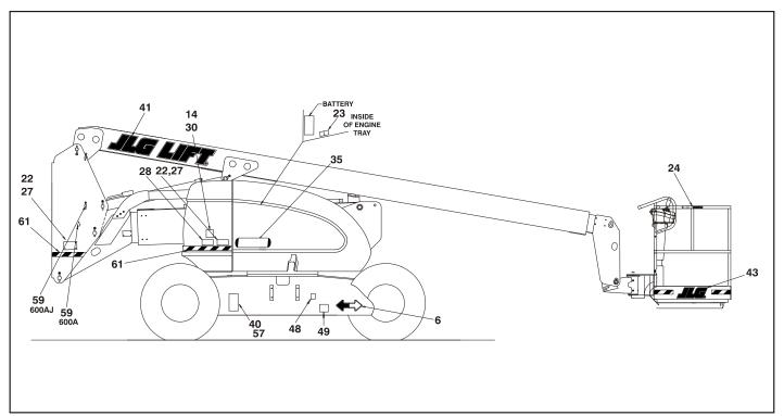
Figure 4-12. 600A & 600AJ Decal Installation - Sheet 2 of 4
