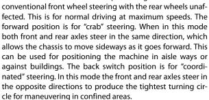
To re-synchronize the front and rear axles, position the rear drive wheels to the forward drive position by selecting either crab or compound steer, then select front steer (center switch position) to operate the normal steering function.
