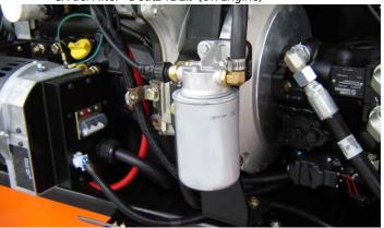
Lube Point(s) - Replaceable Element Interval - Change in accordance with engine manual
