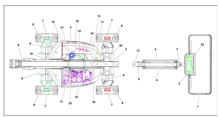
Figure 2-5. Daily Walk-Around Inspection Diagram - GM 3.0L
