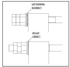
Figure 6-1. Bolt-On External Fall Arrest Cable Tension
