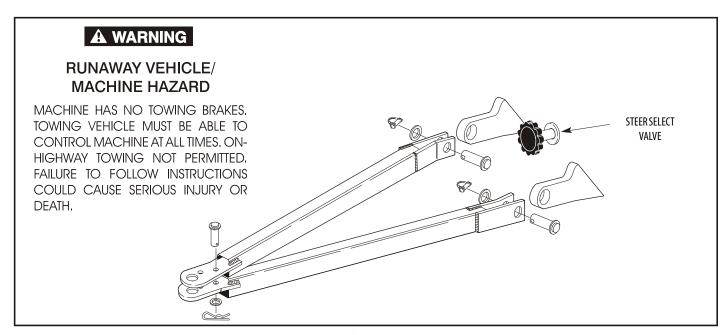
**Figure 4-8. Towbar Connecting Points**
