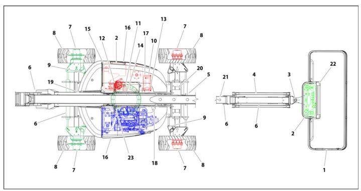
Figure 2-4. Daily Walk-Around Inspection Diagram - Deutz TD2.9
