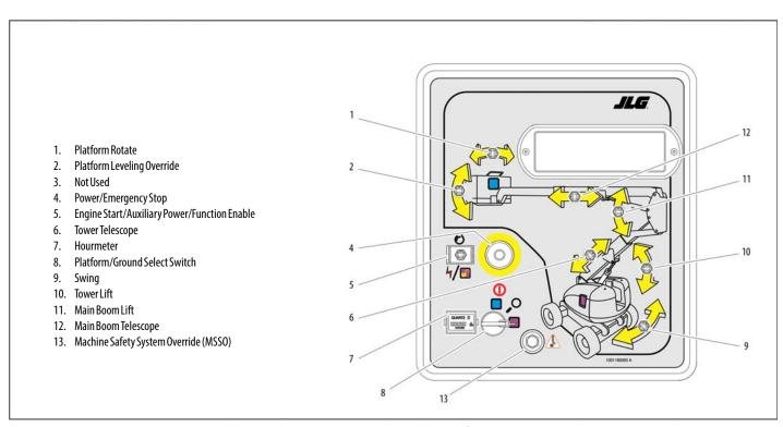
Figure 3-4. Ground Control Station - 600A with Machine Safety System Override (MSSO) (CE Only)
