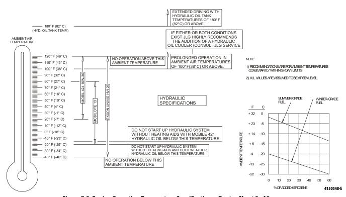
Figure 7-3. Engine Operating Temperature Specifications - Deutz - Sheet 2 of 2
