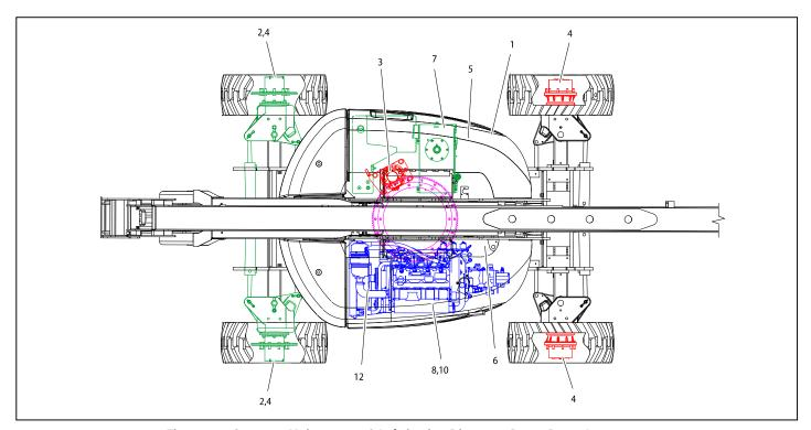
Figure 7-6. Operator Maintenance & Lubrication Diagram - Deutz D2011L04
